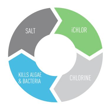
Once the chlorine has finished purifying the pool of contaminants, it reverts back into dissolved salt and the cycle repeats.
